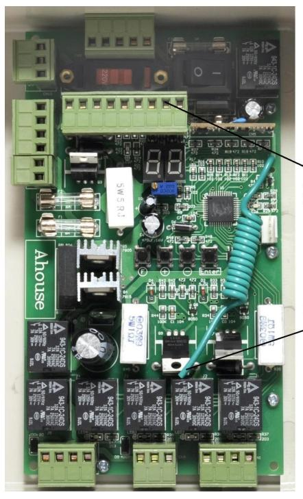
GND wire connects here. The plug can be lifted off to attach the wires and replugged.
